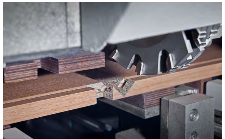
NOTCHING FOR DRAWER SLIDES & HARDWARE
